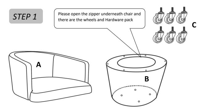
> Position the product bottom-side up and screw the base and wheels into the predrilled holes
